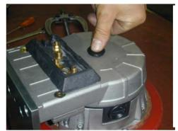
Insert sealing plug into borehole
