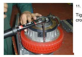
Tighten wheel bolts crosswise with 16Nm
