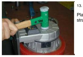
Place brush flange and drive in straight onto the engine shaft
